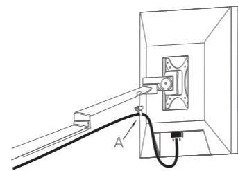
Remove cable clip (A) from the arm, thread cables, install cable clip on the arm again.
